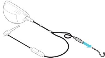
2. Pull out the USB connector at both ends of the probe cord from the Apex Connect Unit and file holder B.
